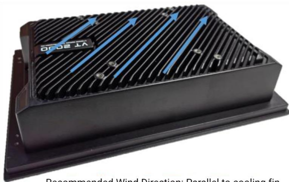
Recommended Wind Direction: Parallel to cooling fin Recommended Wind Speed: \geq 0.7 m/s
