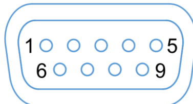
Figure 3-9 DB9 Male Connector
