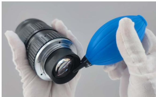
Figure 2-1 Cleaning by Rubber Dust Air Blower
