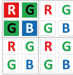
Figure 11-11 Horizontal/Vertical Binning 2 × 2 (Color Device as an Example)
