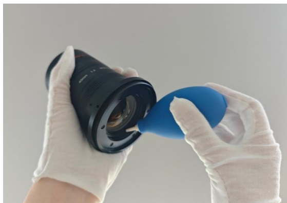
Figure 2-1 Cleaning by Rubber Dust Air Blower
