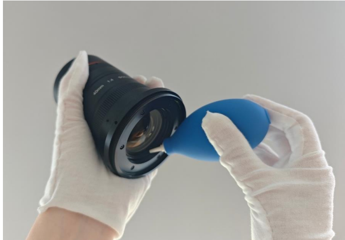
Figure 2-1 Cleaning by Rubber Dust Air Blower
