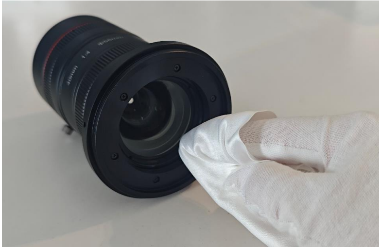
Figure 2-3 Cleaning by Lens Cleaning Paper
