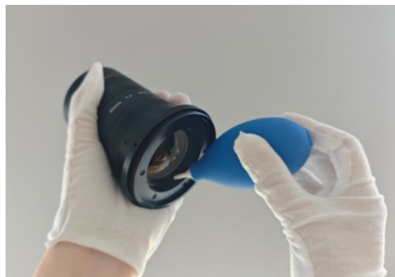
Figure 2-1 Cleaning by Rubber Dust Air Blower
