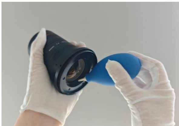
Figure 2-1 Cleaning by Rubber Dust Air Blower
