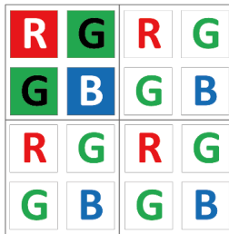
Figure 11-11 Binning Horizontal 2 and Binning Vertical 2
