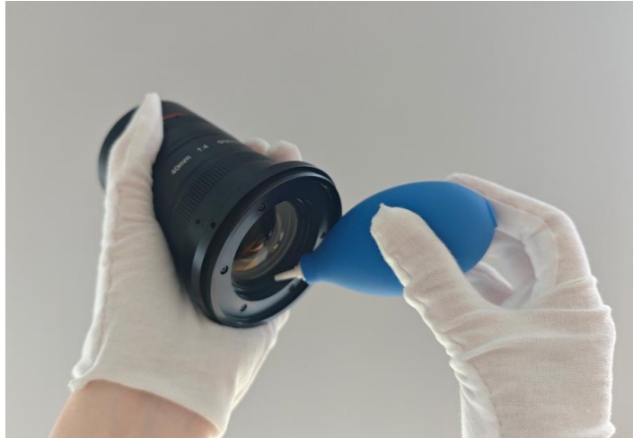
Figure 2-1 Cleaning by Rubber Dust Air Blower
