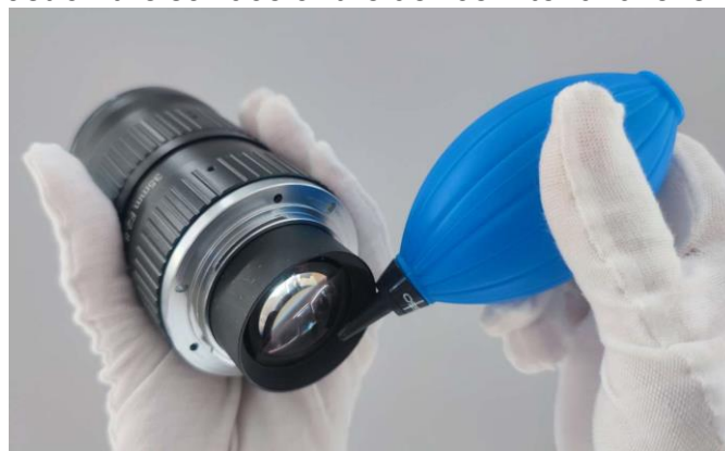
Figure 2-1 Cleaning by Rubber Dust Air Blower
