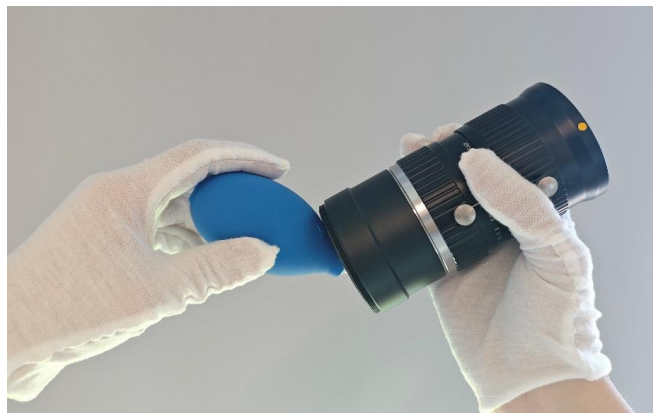
Figure 2-1 Cleaning by Rubber Dust Air Blower
