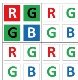
Figure 12-8 Horizontal/Vertical Binning 2 × 2 (Color Device as an Example)
