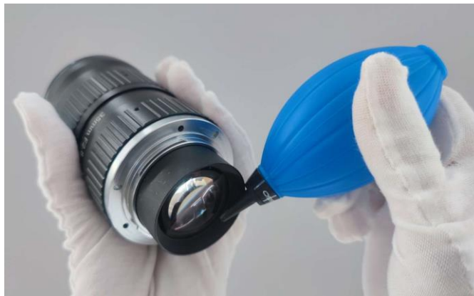
Figure 2-1 Cleaning by Rubber Dust Air Blower
