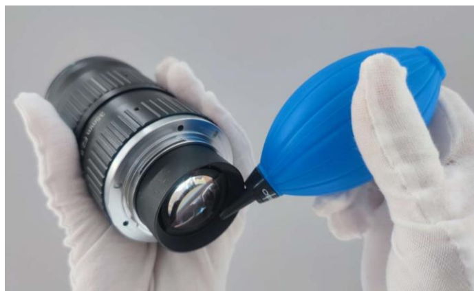
Figure 2-1 Cleaning by Rubber Dust Air Blower
