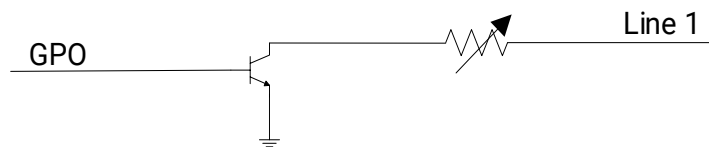
Figure 7-3 Internal Circuit of Output Signal
