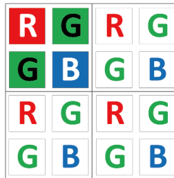
Figure 11-11 Horizontal/Vertical Binning 2 × 2 (Color Device as an Example)
