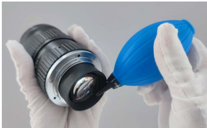
Figure 2-1 Cleaning by Rubber Dust Air Blower
